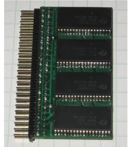
Note that the Cypress data sheet says 90mA is the maximum current at the maximum speed and 100% duty cycle, a condition that will be rare on the home-built computers this is intended for. Even then, it will be for the one SRAM chip that is active at a time, while the other seven are in standby. All eight will be in standby in those cycles in which I/O or anything else in the memory map is being accessed.
