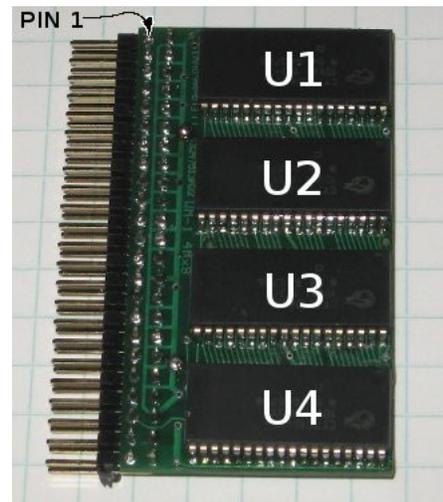
So OE0\ and WE0\ go to the four ICs on the top end of the module, and OE1\ and WE1\ go to the four ICs on the bottom end of the module.
