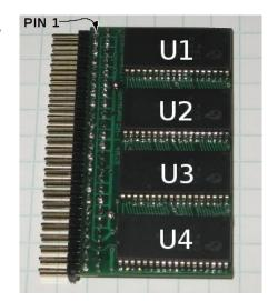
So OE0\ and WE0\ go to the four ICs on the top end of the module, and OE1\ and WE1\ go to the four ICs on the bottom end of the module.
